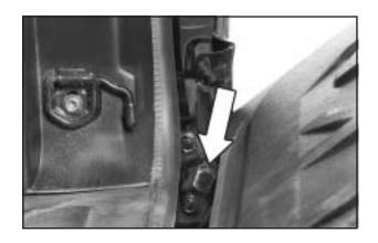
Raise the tailgate at a slight upward angle, pull back on the tailgate at the right edge so it releases from the block hinge and then move the tailgate to the right to release the left edge.
